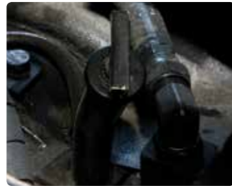
Easy Maintenance Oil Check The T/M oil level can be checked easily without any disassembly.
